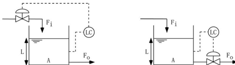
$$A \frac{dL}{dt} = F_i - a\sqrt{L} \quad \text{物質収支式} \quad A \frac{dL}{dt} = F_i - F_o$$
